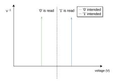
(a) Ideal SLC flash. Nominal voltage levels occur with a probability of 1. Other levels never occur. The probability of a bit error is null.
