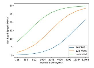
Figure 24 – CPU bound performances on a RAM-like storage device with a 20/MB/s symmetric read/write throughput.
