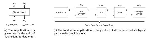
Figure 13 - Amplification can be observed at various levels within the storage stack.
