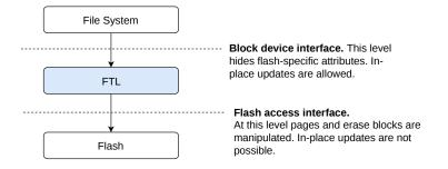
Figure 6 – A flash translation layer (FTL) emulates a block device on top of a flash memory.
