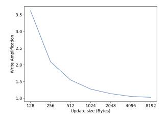
Figure 16 - Write amplification caused by metadata update for various update sizes.
