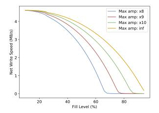
**Figure 21** - The evolution of the average net write throughput as the fill ratio varies, is affected by the maximum allowed write amplification. Throughput values are computed for a hypothetical 256MiB NAND SLC device with a write throughput of 10MB/s, a read throughput of 30MB/s and a 64KiB read cache.
