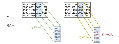
Figure 4 – A block is partially updated through a read-modify-write procedure.
