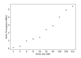
Figure 14 - Write speeds sampled from a class 10 SD card for various write sizes.
