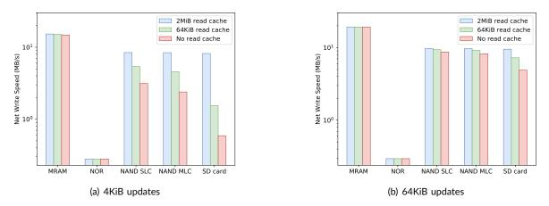
**Figure 19** – Average net random write throughput for various storage devices and read cache configurations for a 256MiB data set.
