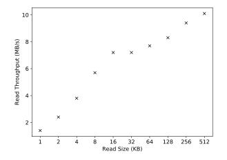
Figure 22 - Read speeds sampled from a class 10 SD card for various read sizes.
