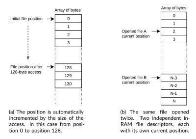
**Figure 1** – The file abstraction and the relation between in-RAM file descriptors and on-disk byte arrays.
