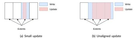
Figure 15 - Partial updates are the result of small and/or unaligned write accesses.
