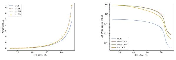
(a) Write amplification versus media fill ratio.
