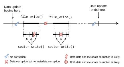
situation is typical of large updates where the data to be written does not fit into a single application buffer.
