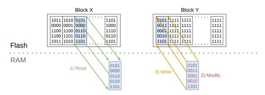
**Figure 7** – A copy-on-write (COW) update as performed by an FTL. In this case, the 3<sup>rd</sup> page of block X is updated into the 1<sup>st</sup> page of block Y.
