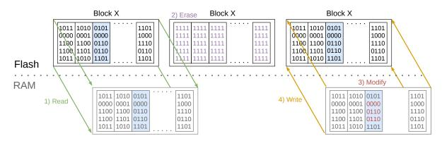
Figure 5 – The third page of block X is updated in-place using a straightforward read-erasemodify-write approach.
