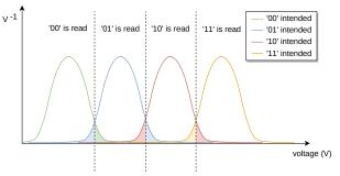
(d) MLC flash. Voltage levels are closer than SLC levels, density functions overlap considerably. The probability of a bit error is significant.
