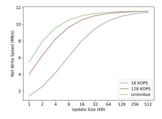
Figure 20 - On RAM-like devices, performances can be limited by system-level bottlenecks.
