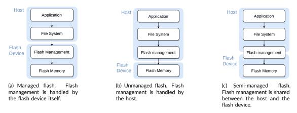
**Figure 9** – Various distributions of the flash management workload between the host and the flash device.
