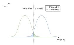
(c) Used SLC flash. The variance is high, density functions overlap considerably. The probability of a bit error is significant.
