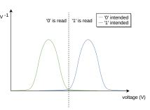
(b) Unused SLC flash. The variance is low, density functions overlap slightly. The probability of a bit error is small.
